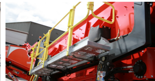
Hydraulically folding maintenance platforms
