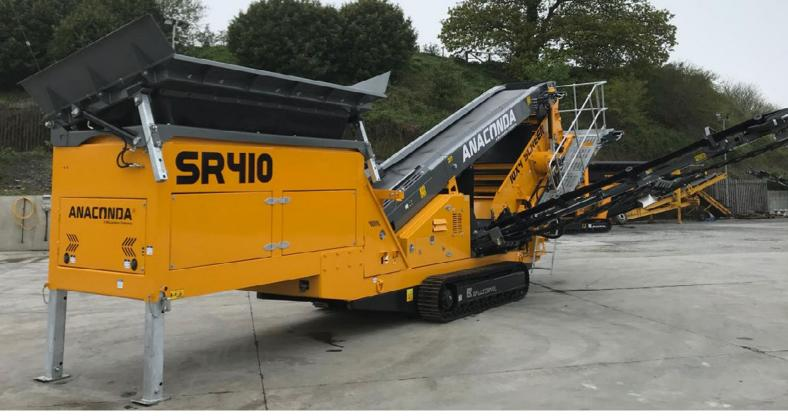
The Anaconda SR Range of Mobile Tracked Finishing Screens have been developed specifically to suit applications where seperating fines is of the upmost importance.
